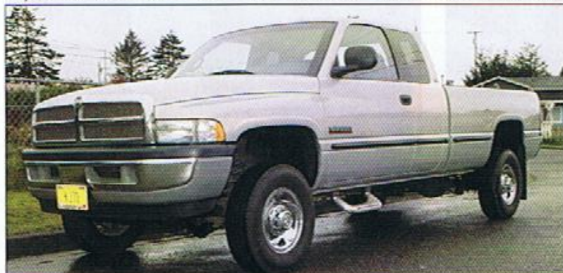
The '99 Dodge 4WD 5.9L Cummins turbodiesel was previously equipped with BD Power Plug-N-Power (50hp increase), a BD exhaust brake, a BD 4-inch exhaust system, and an Advanced Flow Engineering air intake system. The 7,071-mile trip pulling 15,650 pounds averaged 14.9 mpg—about 1.5 mpg better than last trip.
